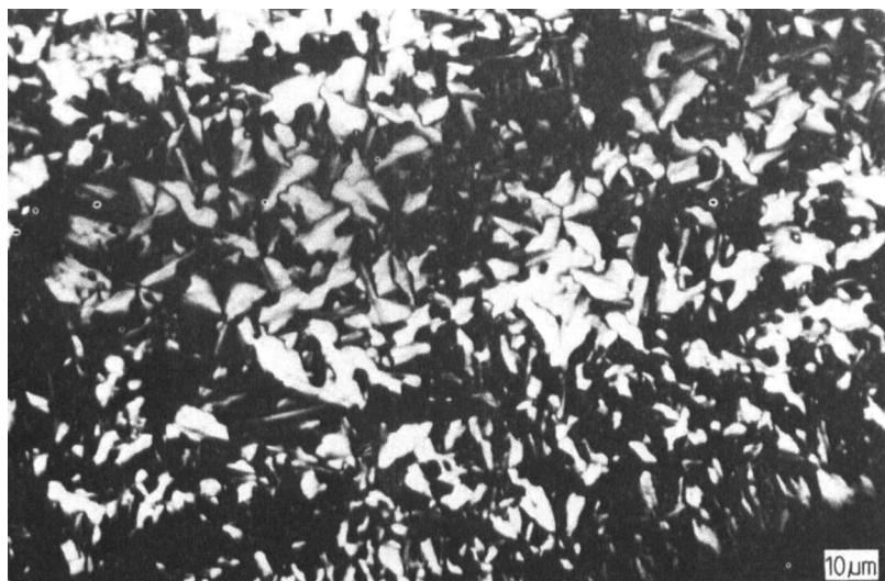
Figure 3. Light microscopy of the side chain liquid crystal with a biphenyl ester as the mesogenic group.
